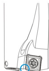
图4 内刃的钻头中心部附近的崩损 FIG. 4 Collapse near the center of the bit at the inner edge
