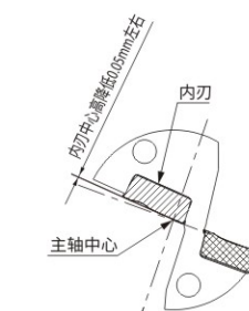
图2 钻头正面图 FIG. 2 Front view of the bit
